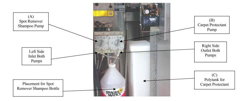
1. Place shampoo products into dispenser assuring that pick-up tube and weight extend to the bottom of the container. Place one gallon Spot Remover Shampoo under Spot Remover Shampoo pump (A). Place Carpet Protectant into the Polytank (C) by Shampoo pump (B). Polytank can be filled without removal from vacuum. Capacity appx. 1.8 gallons.
