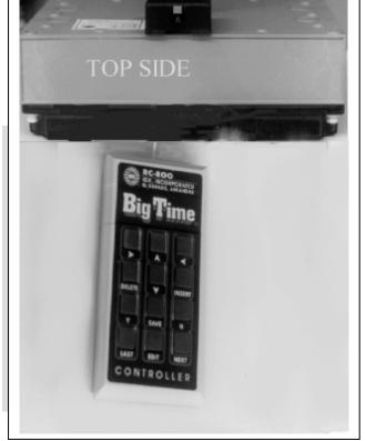
" $\blacktriangle$ " or " $\blacktriangledown$ " key to change the time. To save the "Cycle Time", press the "Save" key. The timer will confirm this by displaying "Saved".
